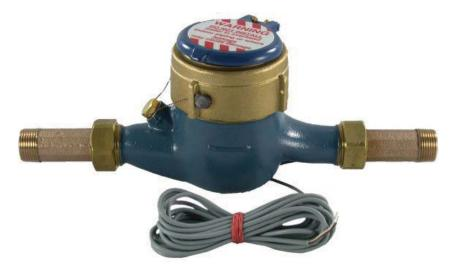
The MDR Series Pulse Meters offer pulse output from a reed switch sensor. This allows the two-wire contact type closure to operate metering pumps, remote indicators and controls.
